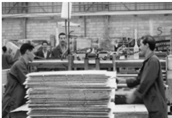
Machine corrugating and gluing paper to make cardboard sheets
